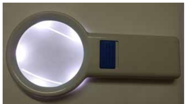
Fig. 1 Biconvex lens mounted with battery operated light emitting devices at the periphery
