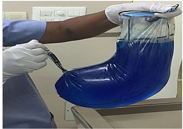
Fig. 12 Bag filled with methylene blue to test for spillage and integrity check
